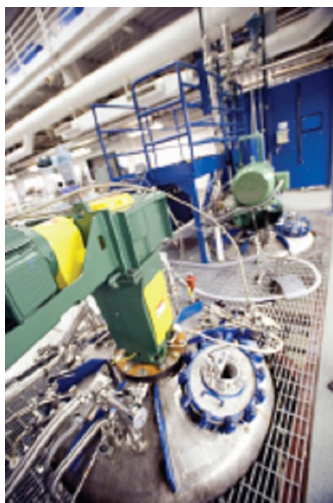
Scaling Up: Genomatica is producing bio-BDO in 3,000-liter fermentation tanks.
